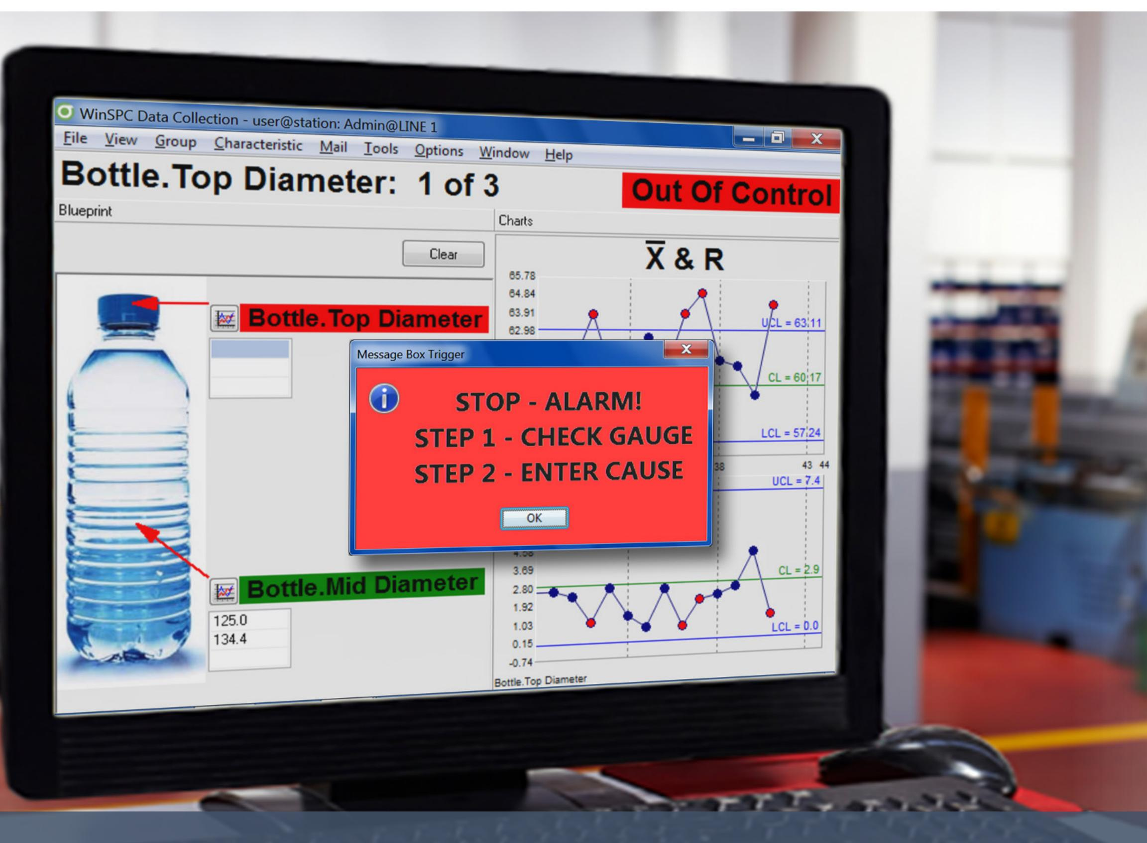
SPC monitors the performance of a process and, using statistics, helps **IDENTIFY TRENDS** and **VARIATION** to prevent the process from going out of control.
